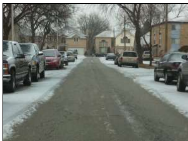
Figure 20: One of our first anti-icing tests clearly shows the benefits of anti-icing. On this day, extremely cold temperatures allowed a minor snowfall to bond to the pavement quickly and cause icing conditions. Areas that were anti-iced had no service issues. Shown here are pictures of two adjacent streets taken within a minute of one another.
