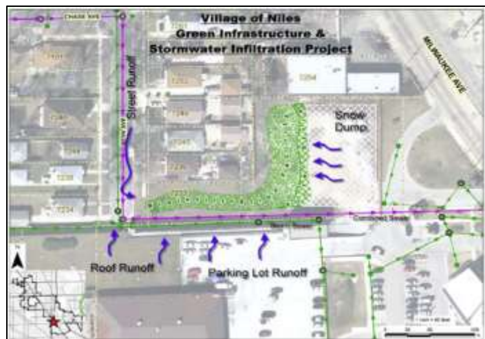
Figure 19: Bioinfiltration Site Plan
